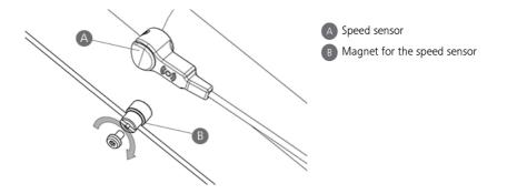
Fasten the mounting screws through the speed sensor and with a cross screwdriver. Tightening the speed sensor onto the frame. Torque requirement: 1.5-2 N.m. (Note: Please make sure the gap between the speed sensor and the magnetic unit is between 10 and 20 mm.)
