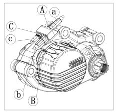
a Male 8 pin connector from EB-BUS to speed sensor
