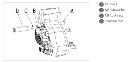
1) Align the three mounting holes of the drive unit with the mounting holes in the bike frame. From the right of the bike frame insert three M8 bolts into the mounting holes in the bike frame and the drive unit.
