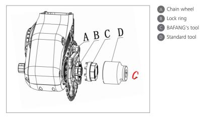
Put the chain wheel onto the spline shaft of the drive unit. Use BAFANG's tool to fasten the lock ring counterclockwise onto the spline shaft. Torque requirement: 35 N.m.
